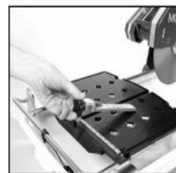
(A) Loosen the Adjustable Cutting Guide retaining thumbscrew
