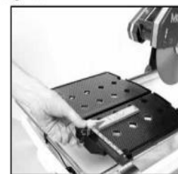
(B) Position the Adjustable Cutting Guide to desired cut length indicated inside the diamond and tighten.
