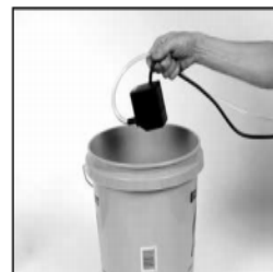
(B) Place the Water Pump in an external container and fill until water completely covers the Water Pump suction
