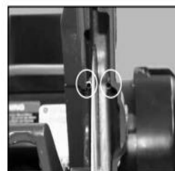
(D) Verify proper cooling flow on both sides of the blade (See Maintenance Section to increase/decrease flow)
