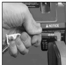
(A) Connect the Cooling Transfer Tube to the inlet connection of the Blade Guard
